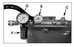
Safety Valve (C): If the unloader valve does not release pressure when tank reaches "blow-off" pressure, the safety valve will protect against high pressure by "popping off" at its factory set pressure (slightly higher than the pressure switch blow-off setting).
